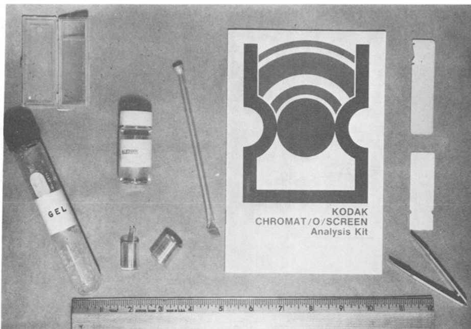
FIG. 3—The TLC items pictured are, from left to right, plastic developing chamber, prepared gel stored in screw-top test tube, acetone, 1- \mu l pipets and holder, instruction booklet, scraper, chromatographic sheet, and plastic forceps. Standard items such as spatulas, labels, vials, and tissue wipes are not shown.
